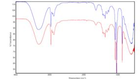
Fig 5. FTIR-ATR of the ethanol obtained from waste coffee (blue) and SRM 2900 Ethanol 95, 6 % by mass (red)
