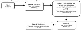
Fig 2. Purification process of crude ethanol obtained from waste coffee industry
