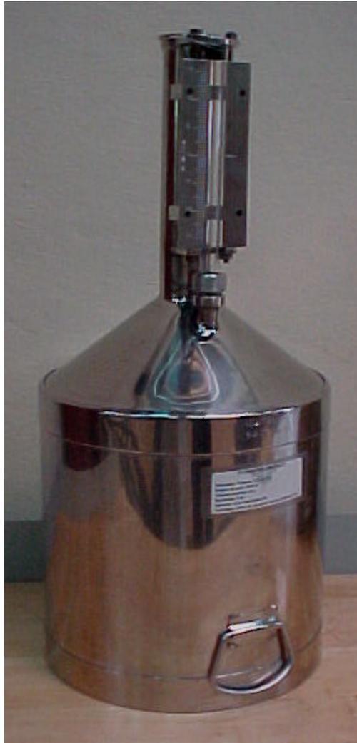
Figure 1.- Transfer standard for volume comparison at 20 L.
